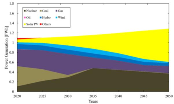
**Figure 2.** The power generation mix in \$50 case.
