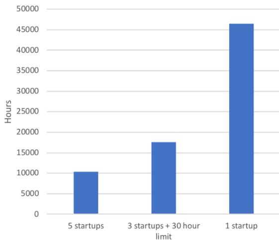
Figure 3: *Expected number of hours that DR is committed during the 88 'key' days modeled. Three types of startup restrictions are: 5 startups, 3 startups and 30 hours of commitment, and 1 startup, all applied over a 5-day time-frame.*
