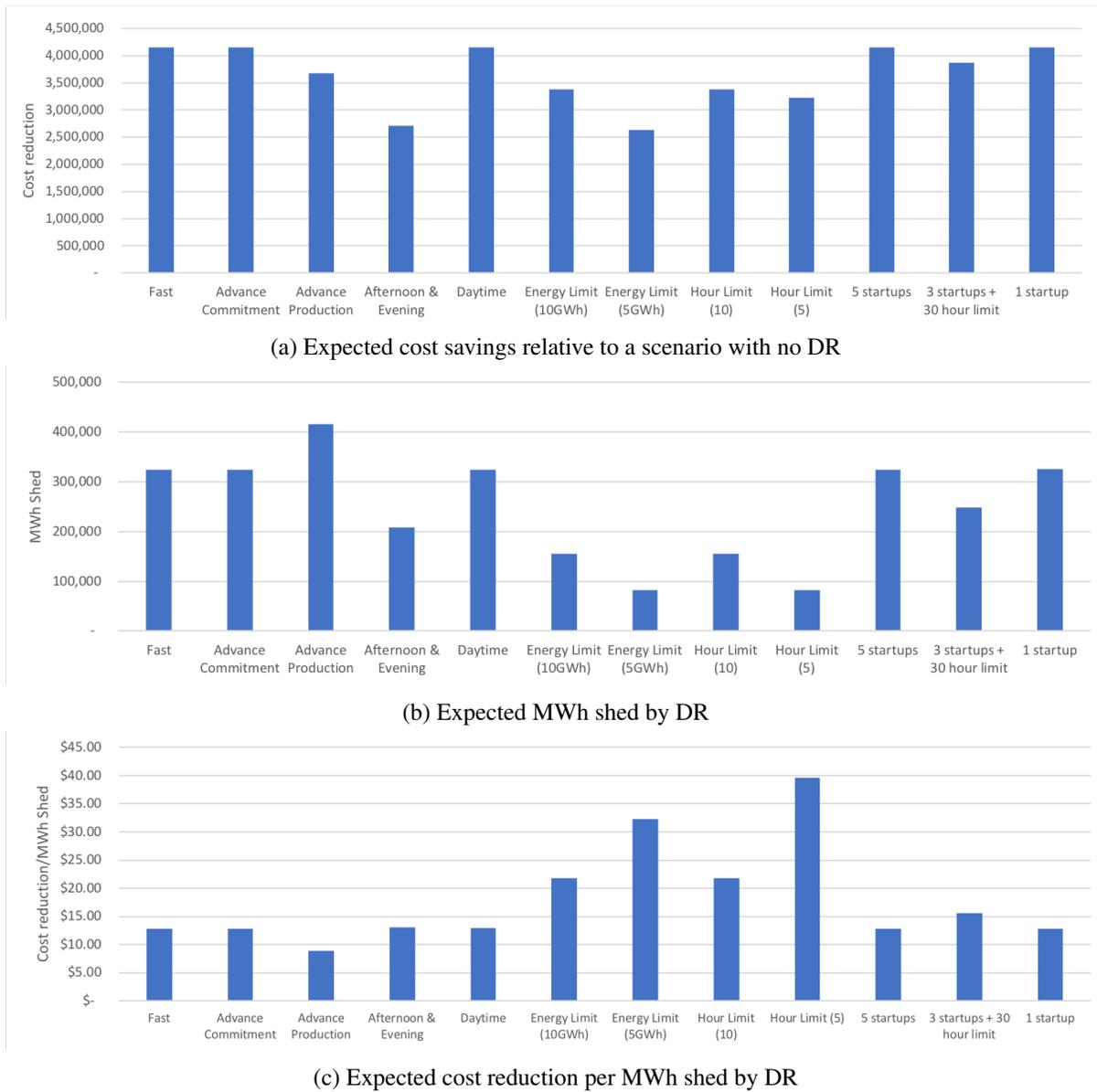
Figure 4: *Effects of introducing DR with various limitations. All values are expected values across 25 demand scenarios, for the 88 most important days simulated. Fast DR, on the left, represents the base case.*
