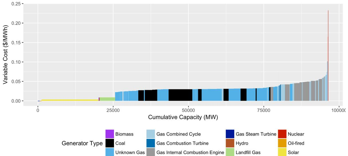
Figure 1: *Supply curve for ERCOT in 2016 as modeled.*
